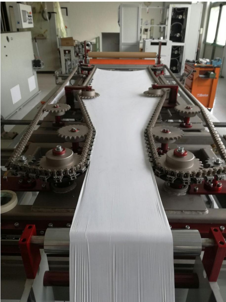
At the same time the transverse stretching takes place through the driving chains equipped with pliers where the tape is hooked. The chains, moving away from each other with a defined angle, allow the stretching for a distance of approximately 1 meter and then they continue parallel to the end of the machine. In this way the resulting tape will be stretched in all sense with the features of a bi-oriented tape.
